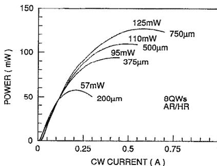
FIG. 4. The cw light-current characteristics of 8 QW lasers having different cavity lengths. The facets are  $\sim 5\%$ –85% AR–HR coated.
