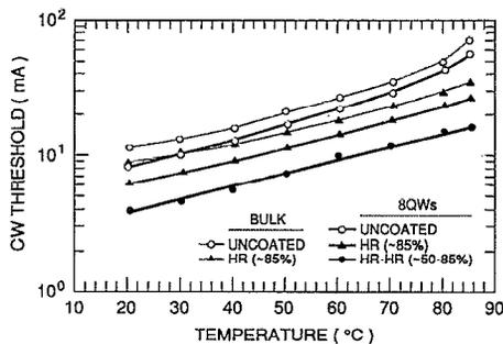
FIG. 3. The cw threshold currents for bulk active lasers and 8 QW lasers, facets uncoated, one side HR coated and both sides HR coated.
