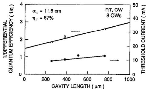
FIG. 1. The inverse of quantum efficiency and cw threshold current of the 8 QW lasers as a function of cavity length.
