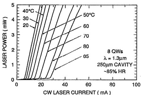
FIG. 2. The light-current characteristics of a typical 8 QW laser measured CW up to 85  $^\circ\text{C}$ .
